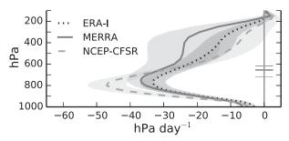
FIG. 12. Sahel region-mean JAS profile of vertical velocity in three reanalysis products. Shaded range denotes plus and minus one standard deviation. Horizontal lines on the vertical axis denote the vertical centroid over the 100–1000-hPa range of the corresponding dataset.
