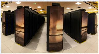
$\approx$ 72K cores = 4536 (nodes)  $\times$  16 (cores) and each core with 2Gb memory 16 Pb parallel file system
