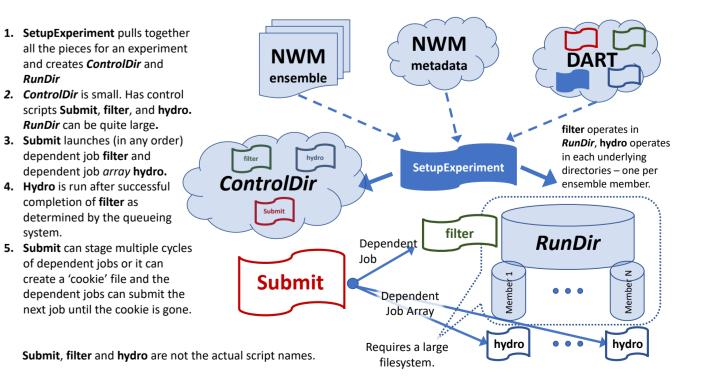
**Figure 10:** Schematic of the workflow of WRF-Hydro and DART. Separate jobs perform the assimilation and a Job Array is used to run the ensemble of WRF-Hydro instances. Each job can be tuned for an optimal configuration. Since each job runs for a very short time, the jobs may backfill. The queueing system takes care of the job dependencies and automatically resubmits the next job in the series.
