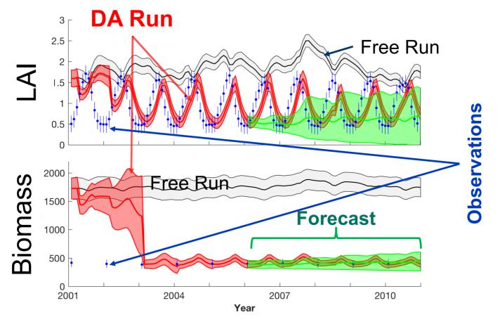
**Figure 3:** This experiment highlights a study in a semi-arid region in New Mexico. Monthly LAI and annual biomass observations are able to provide a much better representation of the sesaonal cycle and accurate initial conditions for forecasting. The impact persists for years for different C pools.
