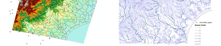
**Figure 8:** Left: The test domain 'Matthew' for WRF-Hydro and DART. The domain is approximately 100,000 km<sup>2</sup>. The triangles are at stream gage locations. The LSM runs at ≈ 1 km resolution. Right: A depiction of the Stream Order.
