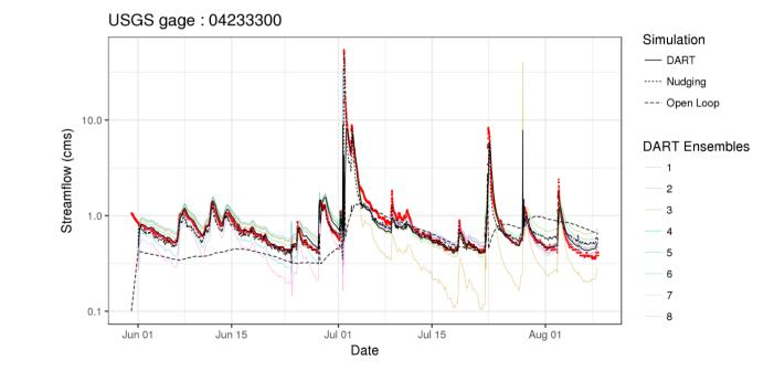
**Figure 9:** The result from a test experiment on a 'channelonly' configuration. This is the verification gage.
