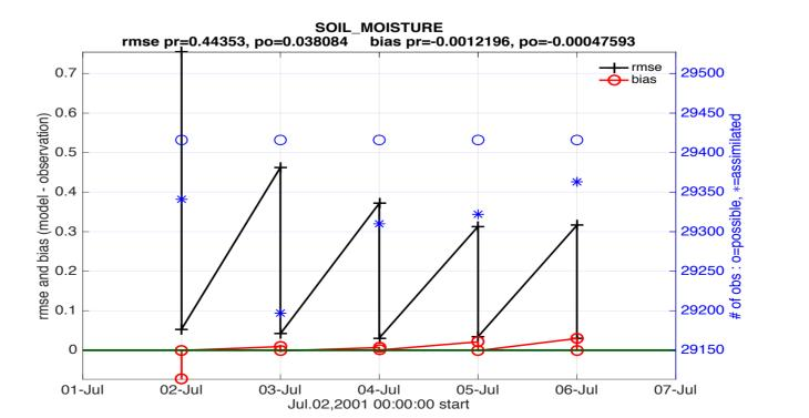
**Figure 7:** The proof-of-concept result for soil moisture in the first layer of CLM. This is a 40 member ensemble.
