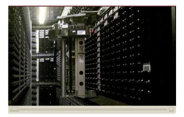
This video shows robots inside NCAR's new AMSTAR digital storage library responding to commands to fetch and mount tape cartridges for reading and/or writing. About halfway into the video, a robot scans the barcode labels on tapes within the library as part of the initial tape inventory process. (©UCAR.) News media terms of use\*
