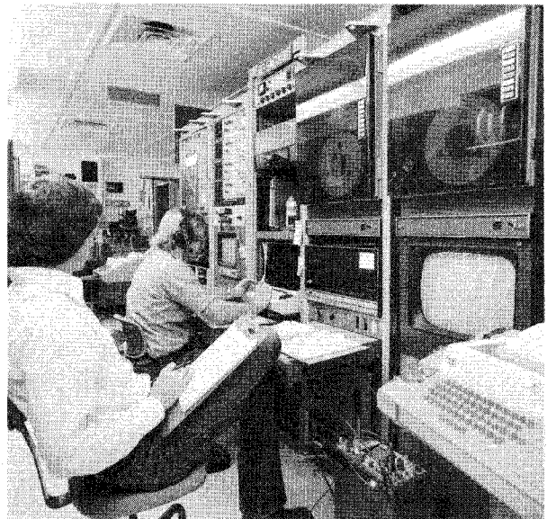
Figure 7c. Ackley Smith (with headset) and John Merrill check out the Data Acquisition and Display System (DADS). DADS is the primary operational data recording and display unit capable of displaying S-band reflectivities in various selectable formats on the TV monitors in the Operations Room. MINA II is a second independent processing and recording system which records reflectivities at both wavelengths but displays only S-band reflectivity.
