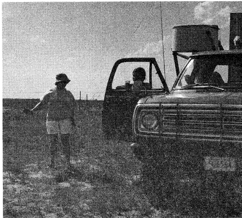
Figure 29b. Nancy Knight (left) and Kathy Kimmel (behind door) await a storm. The NCAR sampling vehicle is equipped with a hail catcher that is used for collecting time-resolved hail samples.
