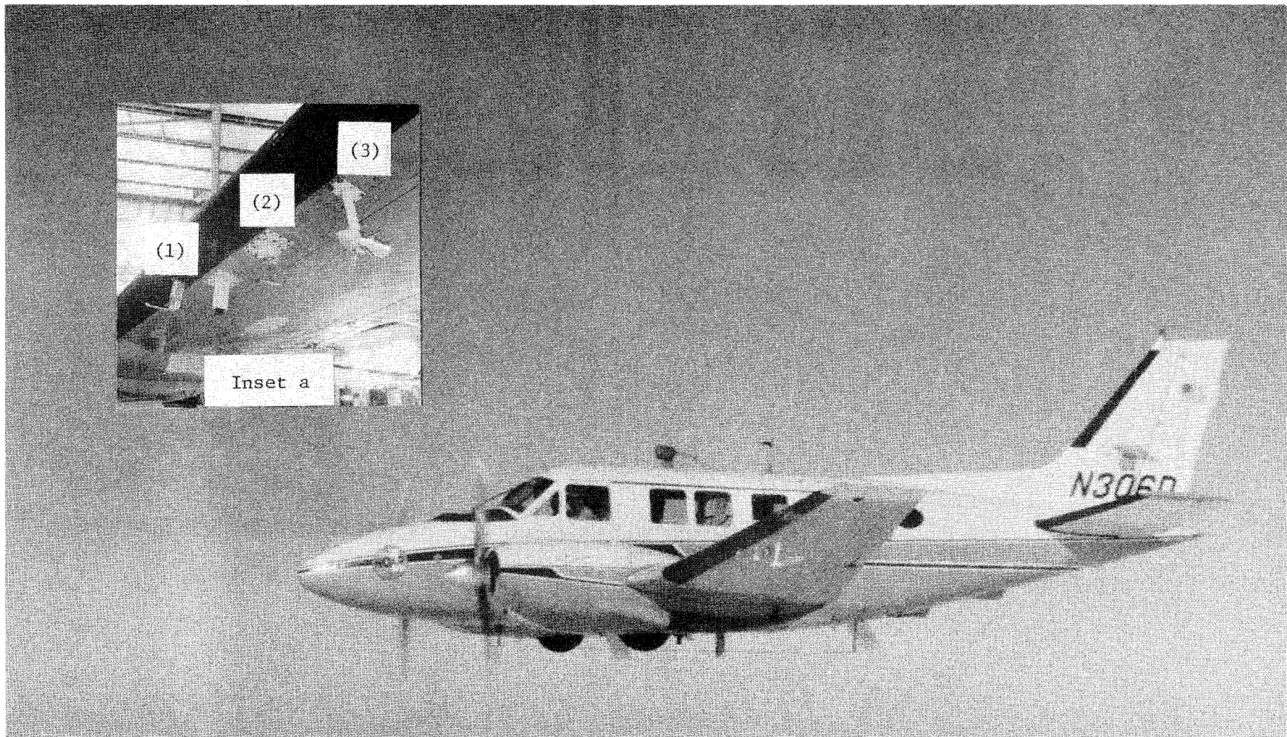
Figure 12. The meteorologically instrumented Beechcraft Queen Air N306D, also operated by the Research Aviation Facility, was used to obtain air motion and precipitation physics data in updraft and inflow regions of hailstorms. Sampling intakes for cloud physics measurements are located on the top of the fuselage. Inset a: Instrumentation mounted beneath the wing included: (1) wing-mounted pitot tube for sensing dynamic pressure; (2) Rosemount total temperature sensor; (3) reverse flow temperature sensor.
