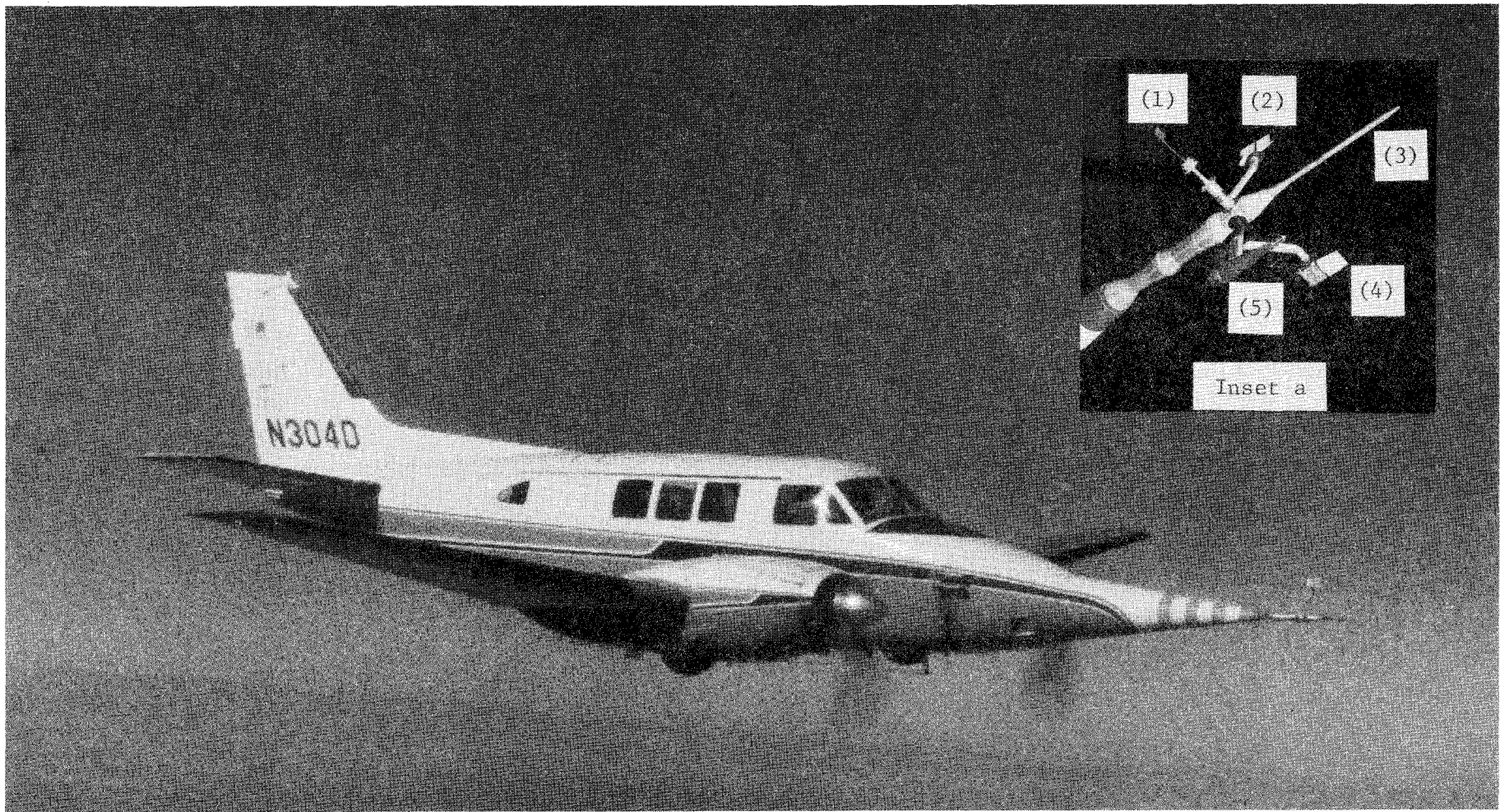
Figure 11. Queen Air N304D, operated by the NCAR Research Aviation Facility, Jefferson County Airport, Broomfield, Colorado, was instrumented similarly to Queen Air N306D. The nose boom carried sensors for determining turbulence and gust parameters. Inset a: (1) rotating angle of attack vane; (2) fixed side-slip vane; (3) probe tip containing sampling ports for dynamic and static pressure; (4) fixed angle-of-attack vane; and (5) fast response temperature sensor.
