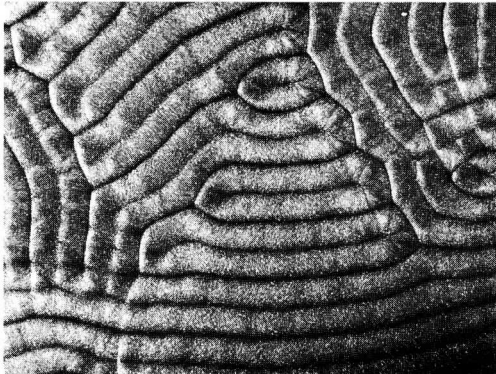
Soon after onset of convection the dominant convective pattern is of long rolls or roll segments.
