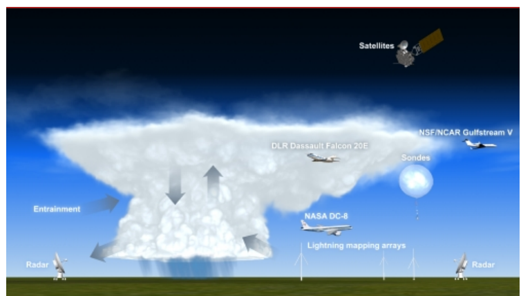
The DC3 field project will deploy a variety of airborne and ground-based instruments to study thunderstorms. (©UCAR. This image is freely available for media & nonprofit use.)
