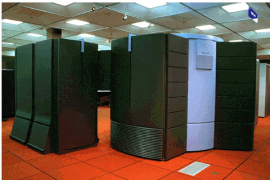
The C-90 weighs in at 256 million words of memory with 5 gigaflops. On the left is the machine's solid-state storage device; at right is its central processing unit.
