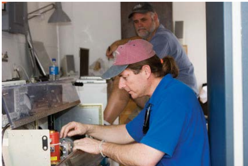
ACD's James Hannigan (left) and Michael Coffey, working in a trailer outside Mexico City, record the absorption of infrared solar radiation in the atmosphere. Such information is used to determine levels of gases in the atmosphere.
