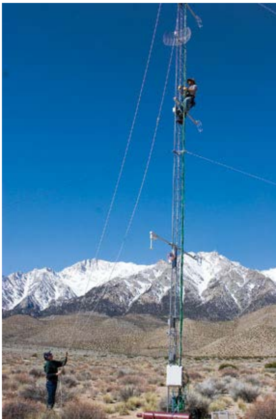
EOL's Gordon Maclean (bottom) and John Militzer remove an antenna from a 110-foot flux profiling tower in the Owens Valley.
