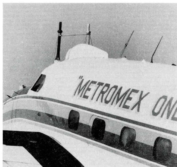
Fig. 3 Axially scattering spectrometer probe (black mast on left) mounted on University of Chicago Cloud Physics Laboratory airplane. Silver probe (to right of spectrometer) is an earlier, prototype scattering probe.
