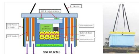
This schematic shows the balloon-based Driftsonde concept. The Driftsonde releases dropsondes, which measure and relay information on wind, temperature, humidity and other meteorological characteristics as they descend through the atmosphere. These data get sent back to the Driftsonde. In turn, the Driftsonde transmits the data to satellites, such as the IRIDIUM Leo satellite, which provides critical information used in near-real time weather forecasting.
