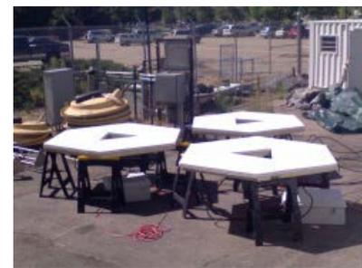
The prototype hexagonal antenna modules of EOL's new 449 MHz wind profiler radar undergoing testing at NCAR Foothills Lab in Boulder.
