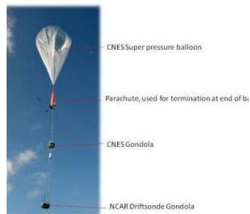
Flight train of Concordiasi balloon just after launch in Antarctica.
