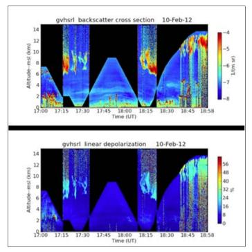
**Figure 5:** During flight operations, HSRL located aerosol layers, the top of the boundary layer, and other features relevant to the measurement strategy.
