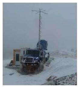
Figure 15: The Center for Severe Weather Research (CSWR) Doppler on Wheels (DOW) radar set up at ASCII.
