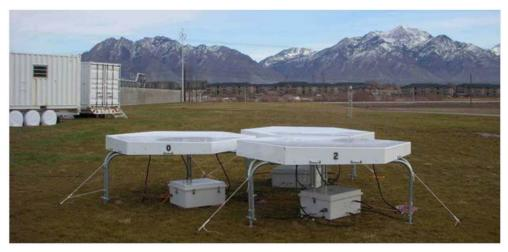
Figure 22: A 3-panel 449 MHz profler system during PCAPS
