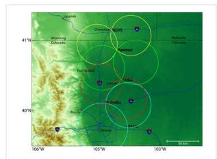
**Figure 25:** The FRONT domain, showing the layout of radars for FRONT overlaid on Front Range topography. Colored circles indicate dual-Doppler lobes between nearby radar pairs.
