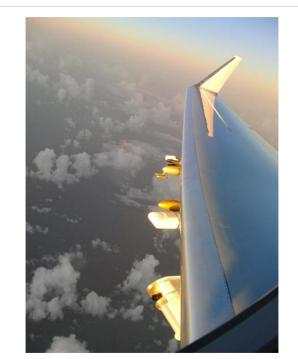
Figure 4: SDI (top), MTP (center) and the 3V-CPI (bottom) instruments mounted on the wing of the NSF/NCAR HIAPER aircraft.
