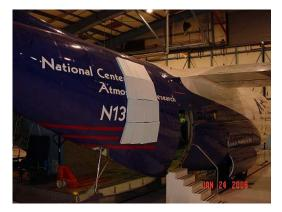
Figure 28: The NSF/NCAR C-130 with a model (styrofoam panels) of the Line Replaceable Units (rectangular elements) and the full sized aperture (the four by four matrix) for APAR.
