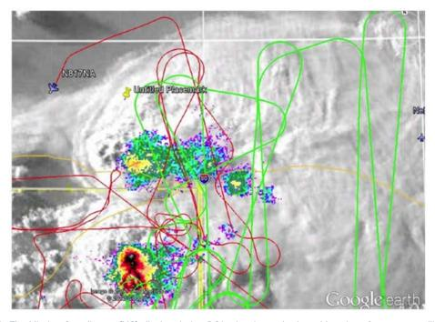
Figure 29: The Mission Coordinator (MC) display during DC3, showing radar based location of storms, satellite overlay of clouds, the GV flight track in green, and the NASA DC8 flight track in red. Items that can be displayed include NEXRAD radar, CAPPI at flight level, research radards, satellite (IR/vis), lightning, (NAPLN/LMS), camera from the GV, flight track with winds, flight plan, and VORs and other navigational points.
