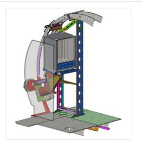
Figure 21: NSF/NCAR GV AVAPS system schematic
