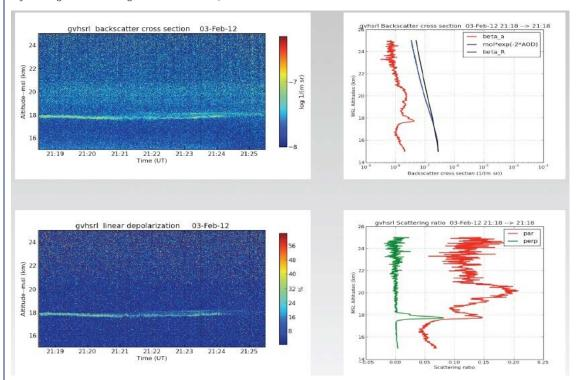
**Figure 14:** Observations of stratospheric aerosols and sub-visible cirrus clouds using HSRL in TORERO. Data from one approximately five minute zenith observation from a flight level above 13 km is shown above. Depolarization was used to discriminate between the non-spherical ice cyrstals of the cirrus clouds and the spherical stratospheric aerosols.
