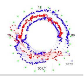
**Figure 3.** Neutral winds observed by HiWind (blue) in both the poleward and equatorward look directions, together with ion velocities observed by EISCAT (red) and neutral winds predicted by the TIMEGCM (green), as a function of local time (LT).
