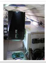
Loaded on the NSF/NCAR Gulfstream V (GV) in downward-looking mode, the High Spectral Resolution Lidar (HSRL) measures microscale aerosols during a research flight.
