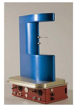
**Figure 3:** The Vertical Cavity Surface Emitting Laser Hydrometer (VCSEL).
