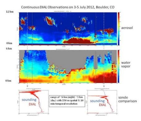
Figure 27: The first continuous observations of the WV DIAL, from NCAR's Foothills Lab.
