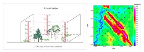
**Figure 23:** Two possible experiemental designs that could use CentNet. The design on the left would study CO<sub>2</sub> advection within a sparse forest canopy using the box budget method with several clusters of multiple-level CO<sub>2</sub> flux towers. The design on the right would employ an extensive array of multiple-level towers to produce a flow map over complex terrain. This map would be used as a validation data set for wind turbine siting models.
