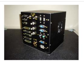
**Figure 2:** The CIMS instrument, developed by Georgia Tech University.
