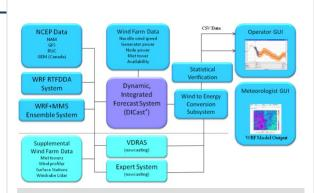
Figure A: Conceptual diagram of the wind energy prediction technology components incorporated into the system configuration.
