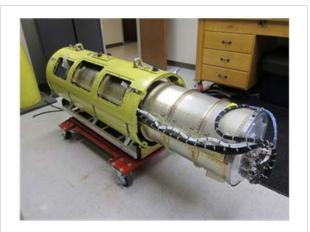
Figure 24: The HIAPER Cloud Radar in its pod configuration.
