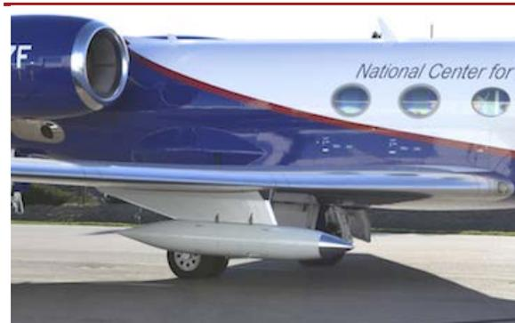
The HIAPER Cloud Radar (HCR) sits in the high-tech pod especially developed to house instrumentation during research flights; the pod sits beneath the wing of the NSF/NCAR Gulfstream V.
