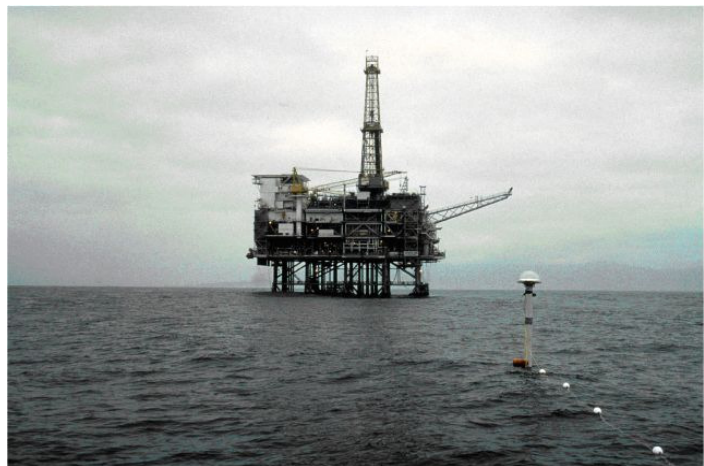
Figure 6. A GPS antenna is deployed on the spar buoy adjacent to the Harvest oil platform west of San Diego. Data from this experiment were used to calibrate the satellite altimeter onboard the TOPEX/POSEIDON satellite.
