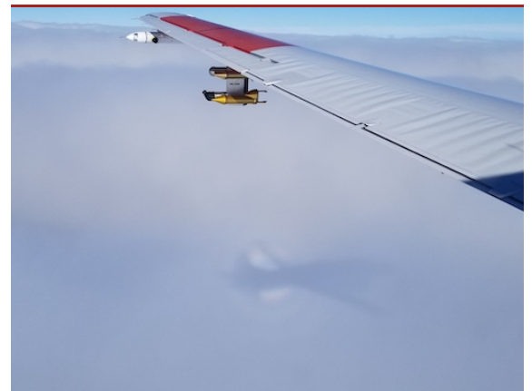
Instruments and sensors are attached to the wing of the NRC Convair 580 to gather data on supercooled liquid water and ice crystals during flight. (Image: National Research Council of Canada)
