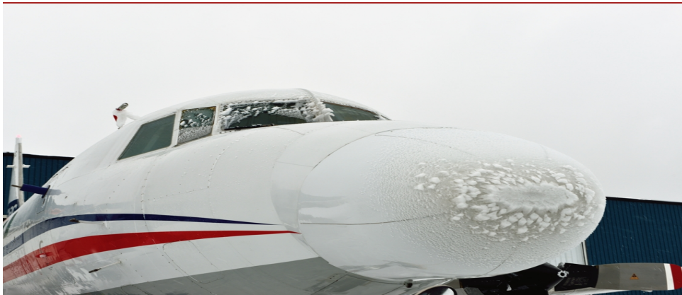
Ice buildup on the NRC Convair 580 can be seen on the aircraft nose and windows after a flight to collect data on ice-prone weather conditions. (©UCAR. Image: Scott Landolt/NCAR)
