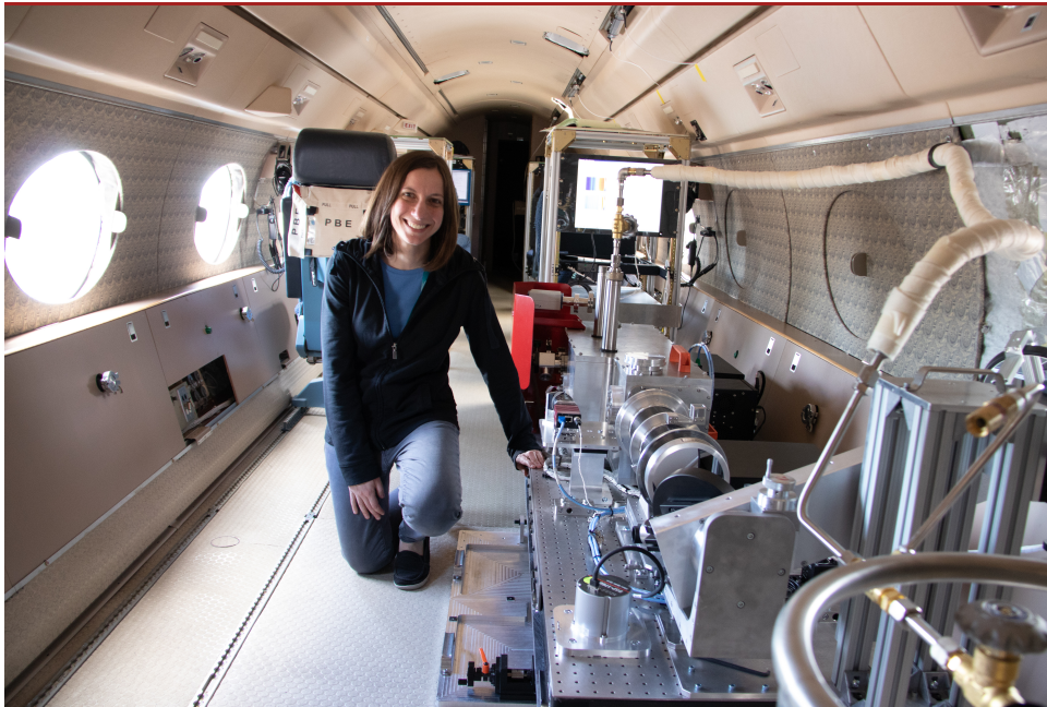
Instrument scientist Jenna Samra kneels next to the Airborne InfraRed Spectrometer (AIR-Spec), an instrument that will be used to view the 2019 South American solar eclipse and measure infrared wavelengths from the Sun's corona. The instrument is mounted on the NSF/NCAR GV research aircraft. (©UCAR. Image: Simmi Sinha)
