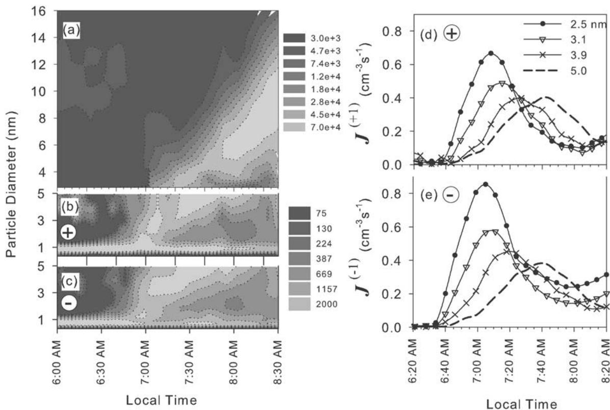
**Figure 10.** Measurements obtained during the new particle formation event on 13 June 2004. Number distributions ( $\Delta N/\Delta \log D_p$ ,  $\text{cm}^{-3}$ ) of (a) total (SMPS), (b) positive (IGMA), and (c) negative (IGMA) particles are shown.  $J^{(\pm 1)}$  ( $\text{cm}^{-3} \text{s}^{-1}$ ) for (d) positive and (e) negative intermediate ions versus time is shown.
