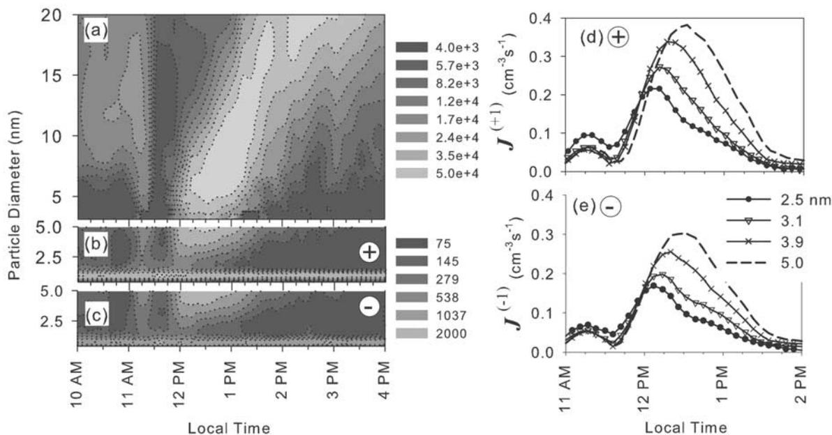
**Figure 9.** Measurements obtained during the new particle formation event on 7 May 2004. Number distributions ( $\Delta N/\Delta \log D_p$ ,  $\text{cm}^{-3}$ ) of (a) total (SMPS), (b) positive (IGMA), and (c) negative (IGMA) particles are shown.  $J^{(\pm 1)}$  ( $\text{cm}^{-3} \text{s}^{-1}$ ) for (d) positive and (e) negative intermediate ions versus time are shown.
