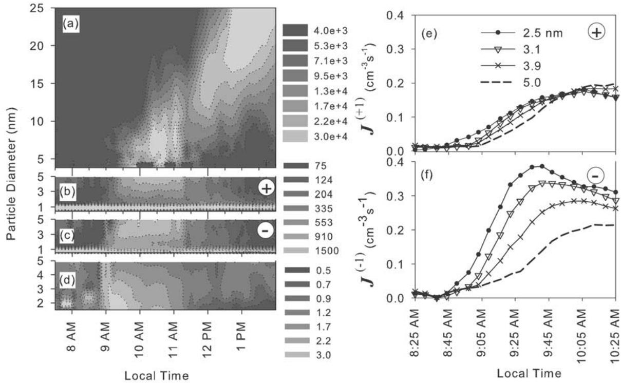
**Figure 11.** Measurements obtained during the new particle formation event on 8 August 2004. Number distributions ( $\Delta N / \Delta \log D_p$ , cm<sup>-3</sup>) of (a) total (SMPS), (b) positive (IGMA), and (c) negative (IGMA) particles and (d) the ratio of positive to negative distribution functions are shown.  $J^{(\pm 1)}$  (cm<sup>-3</sup> s<sup>-1</sup>) for (e) positive and (f) negative intermediate ions versus time is shown.
