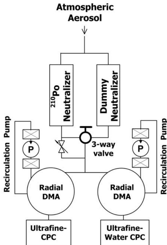
**Figure 2.** Schematic diagram of the dual-SMPS system.
