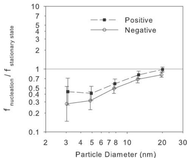
**Figure 8.** Ratio of the average charged fraction during the nucleation hours to the stationary state value for all new particle formation events observed from 15 June 2005 through 27 October 2005. The ultrafine water condensation particle counter was the SMPS detector for all of these data.
