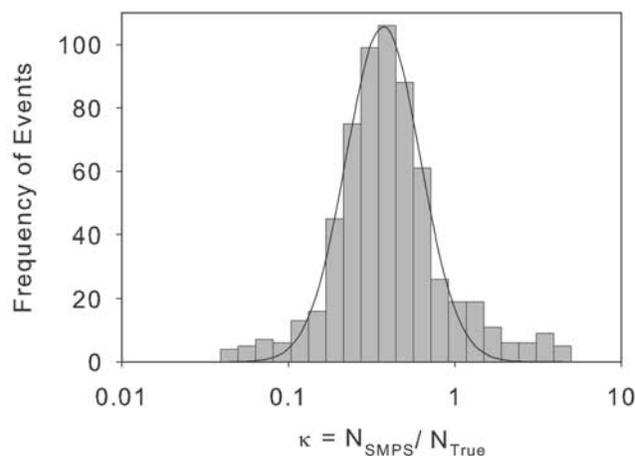
**Figure 4.** Frequency distribution of  $\kappa = N_{\text{SMPS}}/N_{\text{TRUE}}$  obtained by analyzing 4 days of data for which we had simultaneous measurements of the IGMA, SMPS, and dual SMPS.
