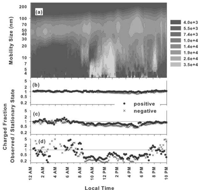
**Figure 7.** Measurements obtained during the new particle formation event on 7 October 2005. (a) Contour plots of the particle number distribution ( $\Delta N/\Delta \log D_p$ ,  $\text{cm}^{-3}$ ) are shown. The dimensionless charged fraction, defined as the ratio of the measured to the stationary state charged fractions, is shown for three size ranges: (b) 11.2–24.5, (c) 5.1–11.2, and (d) 2.4–5.1.
