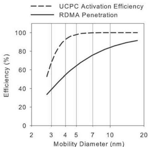
**Figure 3.** Ultrafine condensation particle counter (UCPC) counting efficiency and the radial differential mobility analyzer (RDMA) penetration efficiency obtained from a laboratory calibration using particles in the 2.7 to 17.4 nm diameter range.
