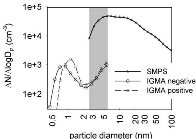
**Figure 1.** Typical particle size distribution measured by the scanning mobility particle sizer (SMPS) and the Inclined Grid Mobility Analyzer (IGMA) during the nucleation event on 1 June 2004. Particle size is defined as mass size [Tammiet, 1995].
