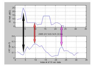
Figure 7: 3D mosaic reflectivity (top, dBZ) and LWC (bottom, gm<sup>-3</sup>) during the second flight leg. Colored arrows indicate the time of each sample discussed previously.
