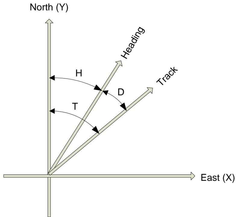
Figure 7.3(a): Definition of heading, drift and track.
