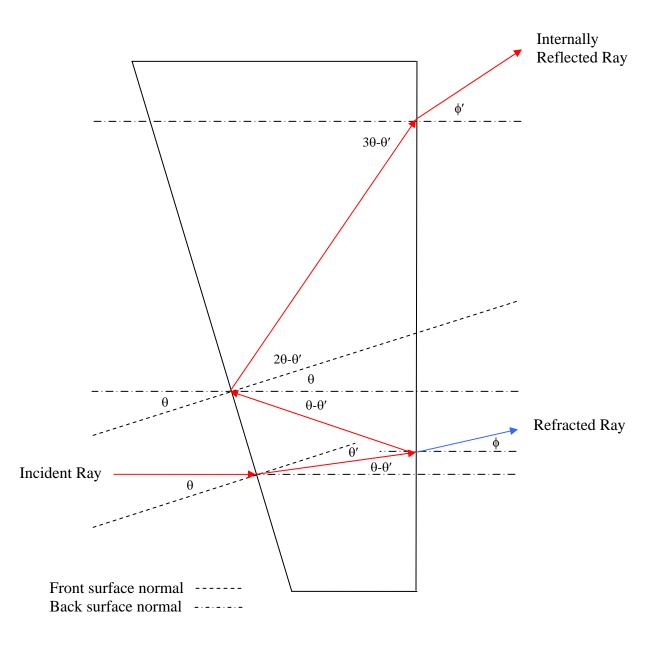
**Figure 1**. Diagram showing the ray paths for the refracted and internally reflected rays in an off axis section of a lens.
