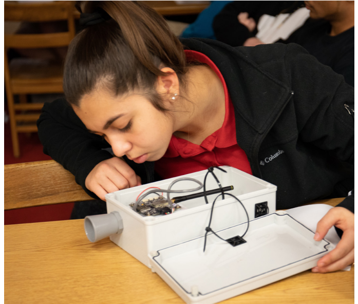
Figure 5. A Jenkins High School student assembling a Smart Sea Level Sensor (courtesy of Russ Clark, Georgia Tech.).
